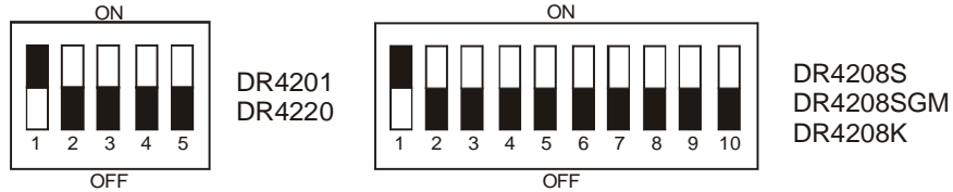
Figure 6: S1 Address DIPs for 4201 and 4220 (Address 1 Selected)
